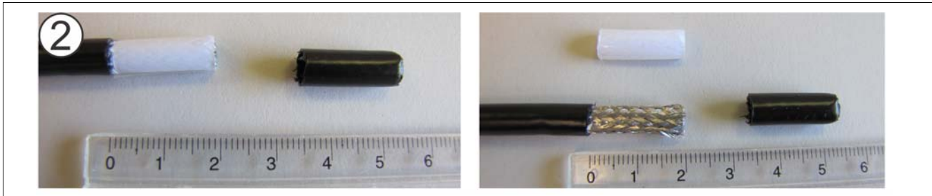
Figure 34: Preparing FlexZone sensor cable step 2
